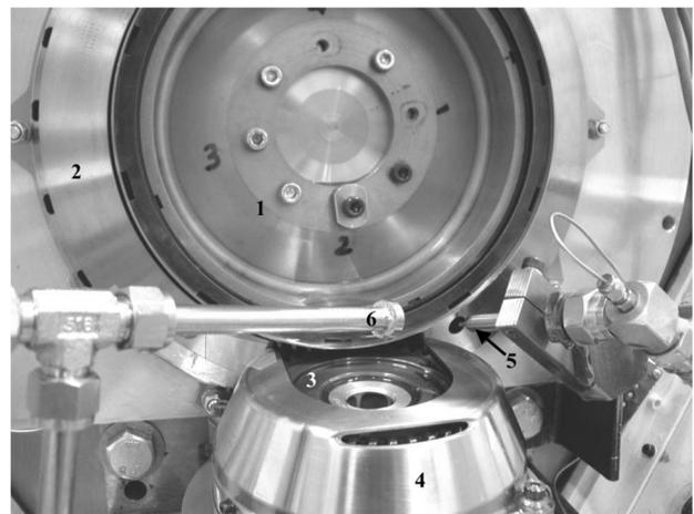
Fig. 3 Shrouded crown gear and pinion. 1. Crown gear; 2. Crown shroud; 3. pinion gear; 4. Pinion - shroud; 5. Into mesh oil jet; 6. Pinion bearing oil jet.
