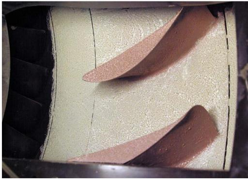
Fig. 21 Oil coating before the surfaces are exposed to the flow
